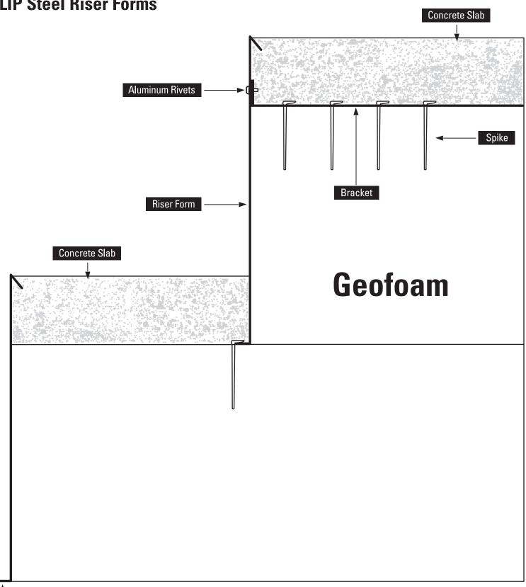
Flange can be in or out at base slab.
